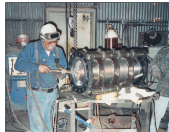
10" DIAMETER MULTI-BELLOWS EXP. JOINT
