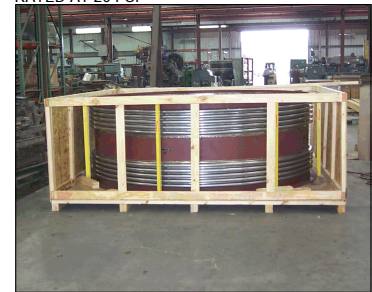
113" DIAMETER UNIVERSAL EXPANSION JOINT RATED AT 20 PSI
